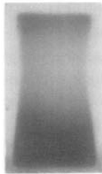
FIG. 4. Photo of a corundum crystal with nonuniform titanium impurity distribution after its thermotreatment in an oxygen atmosphere.
